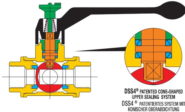
DSS4® PATENTED CONE-SHAPED UPPER SEALING SYSTEM
